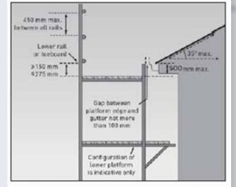
Roof pitch greater than 26° with maximum 35° slope
