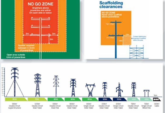
Figure 1: Typical easement widths
